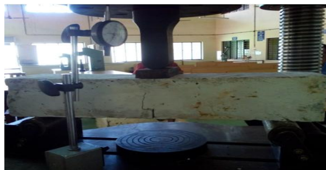
Fig. 5 Loading arrangement for fracture test
